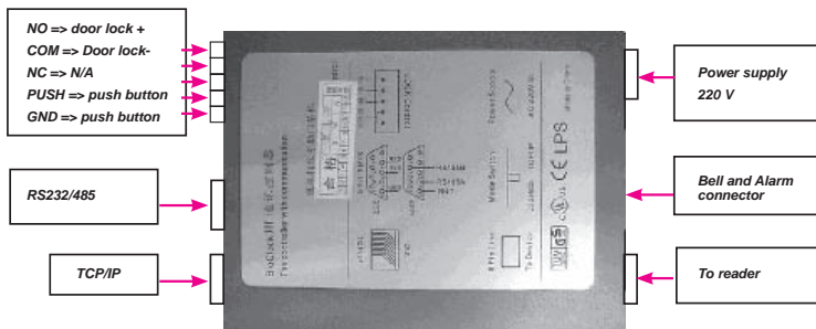
The diagram of an C2 Controller and its points of connections.
